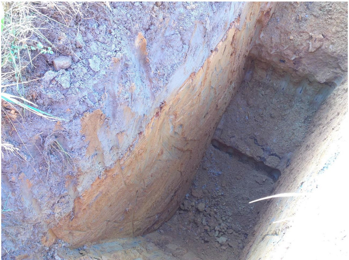
Figure 2. Shallow iron pan over sandstone encountered at test pit 04.
